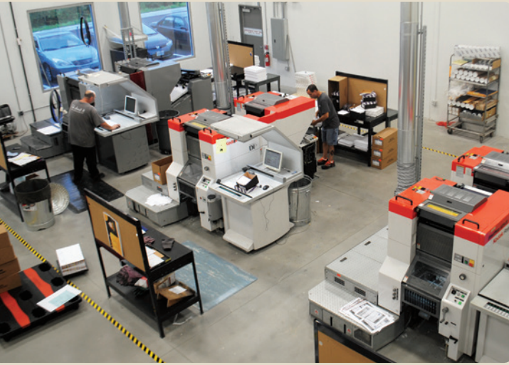
The three DI digital offset presses at Miller's MMP's central production facility, what the company aptly named its "Strategic Factory," provide a "go-to" platform for highly efficient and profitable four-color printing.
