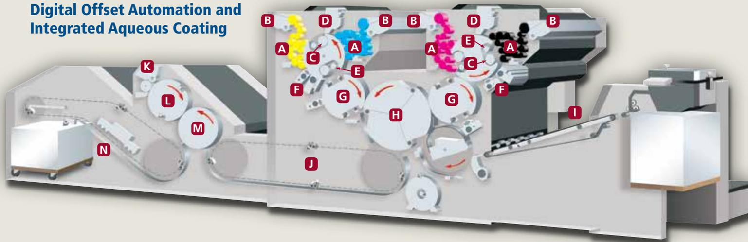
**A)** Waterless offset printing—Ink train has four form rollers. Three chilled rollers significantly reduce toning.
