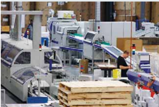
A new Kolbus high-speed perfect binding line keeps up with capacity at Friesens new facility.
