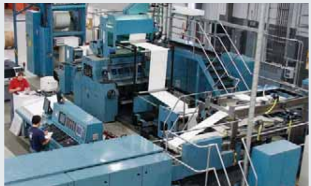
Friesens new Timsons UV book press line operates with a small footprint and less environmental impact.
