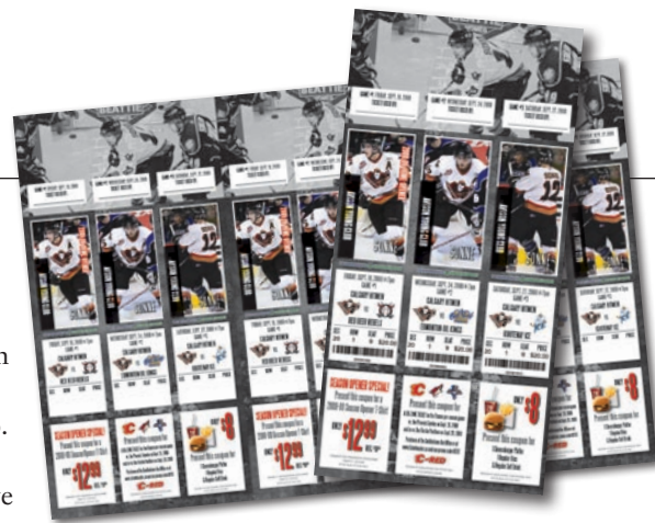
The CRN Group's Presstek 52DI and toner-based presses combine for the best of two worlds: high quality four-color printing with variable data. Tickets for a Calgary hockey team were cost-effectively printed as four-color shells on which variable data was imprinted.
