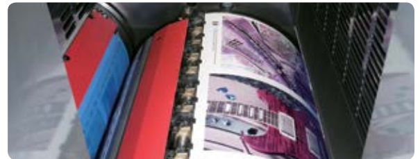
On the central impression cylinder, sheets are inked with all four colors without gripper changes. Precise registration, from the first sheet to the last, is an inherent feature of the Presstek 34DI and Presstek 34DI ECO-UV press design.
