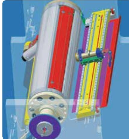
*On-press thermal laser media imaging eliminates variables of off-press platemaking. While the imaging head (at right) is working, cleaning devices (at left) simultaneously prepare the plate for inking.*
