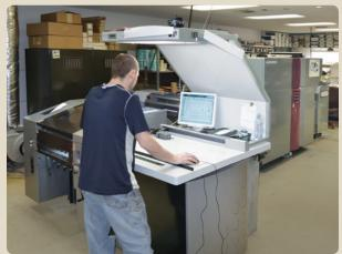
"There just isn't room for a conventional offset press with a coater," says Innovative Ink's Chuck Parkinson. By upgrading their capabilities with a Presstek 52DI-AC, shown above with press operator Justin Schultz, the comapny is able to offer high quality printing with in-line aqueous coating— without expanding or reconfiguring their facility.
