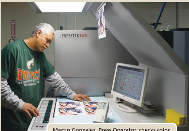
Martin Gonzalez, Press Operator, checks color at the control console of the Presstek 34DI.
