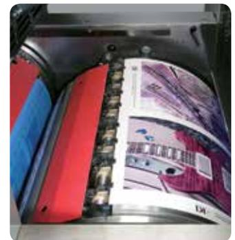
*Left: ProFire Excel imaging and ProFire Digital Media provide an optimised system for fast, accurate, high resolution imaging. Right: On the central impression cylinder, sheets are inked with all four colours without gripper changes. Precise registration, from the first sheet to the last, is an inherent feature of Presstek DI press design.*
